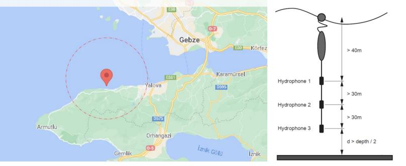
Three hydrophones have been used deployed at three different water depths, at 40, 70, and 100 meter tethered from a support vessel. The three hydrophones were connected to the RTSYS EA-SDA14 data recorder which has been set to sample the hydrophone signal at a sampling frequency 156.25 kHz (24 bit).
